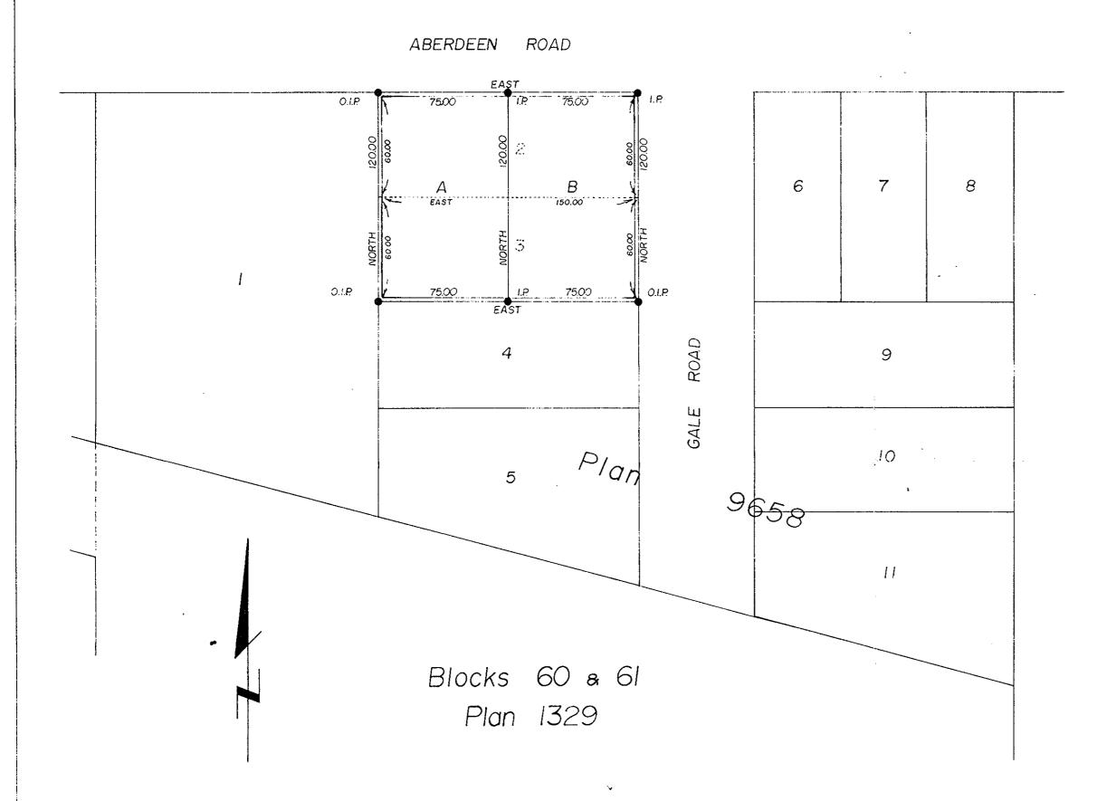
Bearings are astronomic and are derived from O.I.P.s on West boundary of Lot A shown as North on Plan 9685
